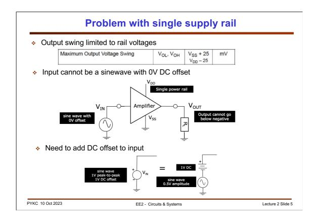
Because we only use only single power supply rail with our op-amp, the output is limited to VDD and GND (VSS). (Note: VDD and VSS are so named because VDD usually supply the drain terminal and VSS the source terminal of the MOSFET transistor inside the op-amp.) For MCP6001, the output swing is within 25mV of the rail voltages.
