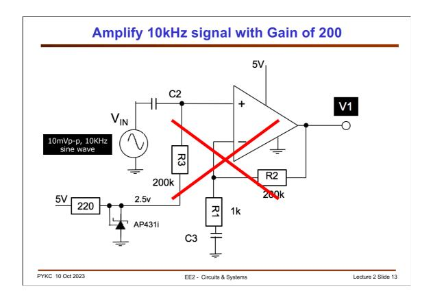
Given the GBP limitation of the MCP6001, the circuit shown here will not work if your signal is 10kHz. Here the gain is expected to be x201. This is beyond the capability of this op-amp. We need a different solution.
