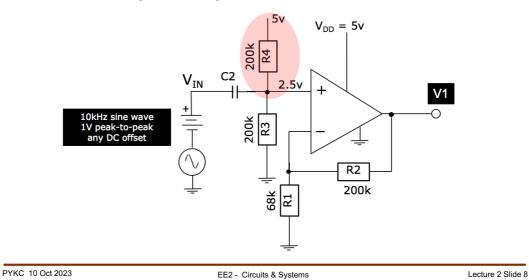
One could try to solve the problem by biasing the V+ input of the op-amp to 2.5V using R3 and R4 as a bias network. Then V+ will always sit on a DC of 2.5V, which is not a bad idea because we now allow a maximum voltage swing to the input.
