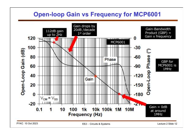
Although the open-loop gain of the MCP6001 at DC (or 0Hz) is very high (at over 100,000), this gain drops off very quickly as the signal frequency is beyond 2Hz. Beyond 2Hz, the gain falls off at a rate of -20dB/decade (i.e. drops by a factor 10 as signal frequency goes up by a factor of 10).
