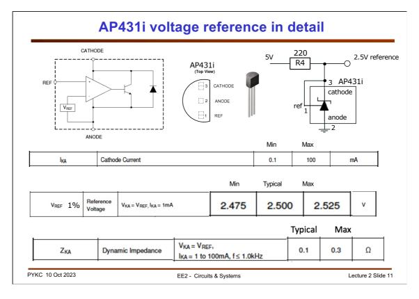
The AP431i actually uses an op-amp internally, with a voltage reference diode as shown here. The output NPN transistor provides high current capability. The diode offers protection if user revise the supply voltage by accident.
