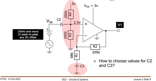
The solution is simply to add C3 in the feedback network of the op-amp.
