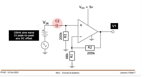
To avoid amplifying the DC offset of any input signal (unless you intend to), one way is to add a capacitor C2 in series with the input as shown in the circuit here.
