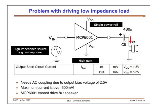
Our final goal is to design a circuit to drive a low impedance load such as an  $8\Omega$  speaker.
